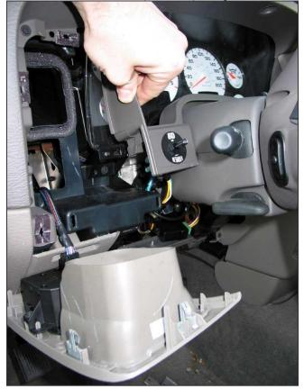
Install switch into drilled hole and secure with lock ring then reinstall dash trim panels by reversing the removal procedure.
