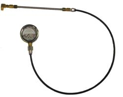
You do not need to measure the air pressure in the system, just the exhaust backpressure. This can be done by installing the pressure gauge on the steel back pressure pipe.
