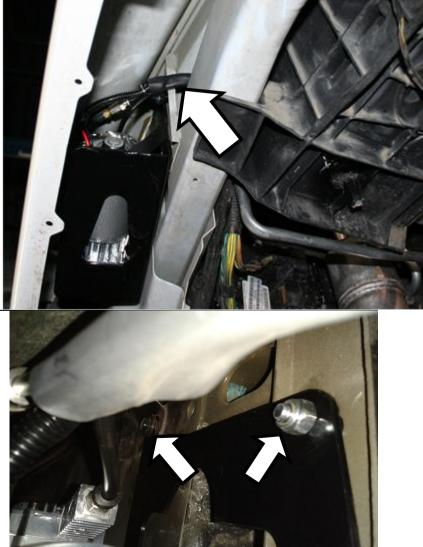
Secure the compressor in place by reinstalling the hood hinge bolt through the compressor bracket. Then install the nut and bolt to hold the front of the bracket.
