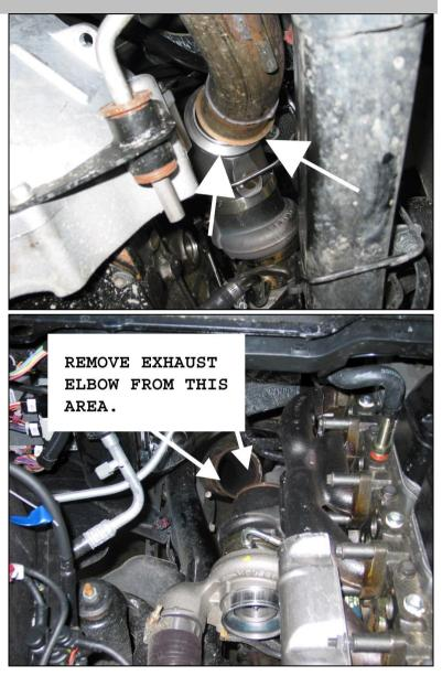
Tighten all clamps that secure the brake to the flanges.
