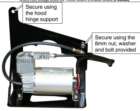
Feed the compressor air lines and wire through the fender into the engine bay, they will be connected later. Lift the compressor into place.
